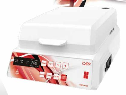
**CAPP** *Rondo* **Incubation Shaker** holds up to 4 micro well plates. A rubber O-ring stabilizes the microplates during shaking and an internal counterbalance mechanism ensures even shaking across all plates. Incubation temperatures stay uniform across all four plates with a tiny temperature variation of only ±0.3°C.
